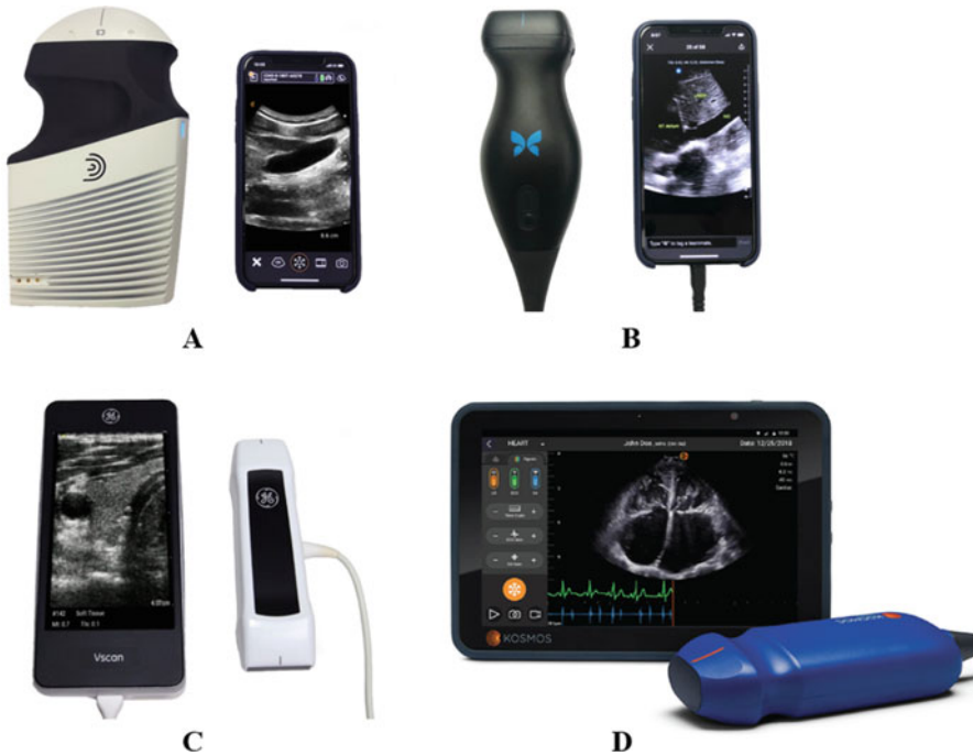
Fig. 12.2 Hand-held ultrasound devices: (a) Wireless probe. (b) Single broad-frequency probe with phone plug-in. (c) Dual-frequency probe. (d) 3-Signal (ultrasound, e-stethoscope, ECG) probe with tablet
