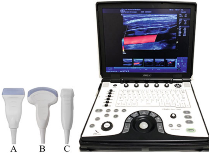
Fig. 12.1 A portable laptop ultrasound system consisting of display screen, console control panel, power source, and storage space for captured images. Also shown are three ultrasound probes that attach to the system and allow scanning of all organ systems relevant to the study of human physiology. (a) Linear array probe. (b) Curvilinear probe. (c) Sector probe
