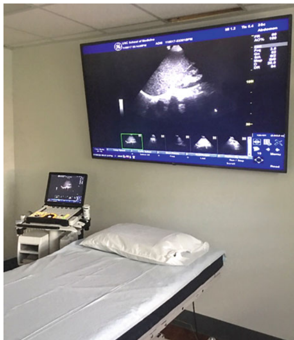
Fig. 12.6 Basic elements of a laboratory scanning station: stretcher, portable ultrasound device, and a large viewing screen
